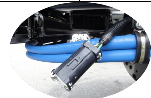
Single connector can be found on LH frame rail near radiator Rev - B
